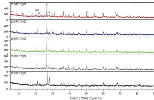
Fig. 5. XRD spectrum. Q: SiO<sub>2</sub> / Quartz, C: CaCo<sub>3</sub> / Calcite, D: CaO MgO 2CO<sub>2</sub> / Dolomite, K: Al<sub>2</sub>Si<sub>2</sub>O<sub>5</sub>(OH)<sub>4</sub> / Kaolinite
