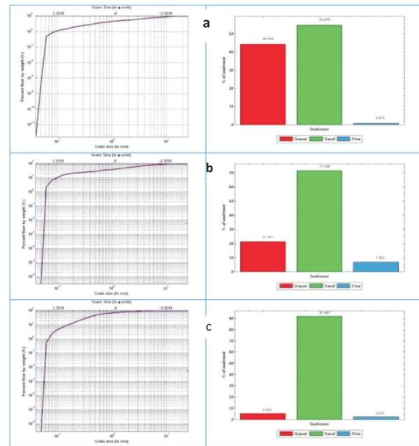
**Fig. 3.** Grain size frequency curves of sand samples from the right bank: a depot samples of the right bank; b depot of the left bank; c paleozoic depot of the right and left banks
